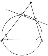
If ABC be any triangle, any line YZ which cuts AC in Y and AB in Z, so that the angle AYZ is equal to the angle CBA, and the angle AZY equal to the angle BCA, is said to be *antiparallel* to the side BC.
